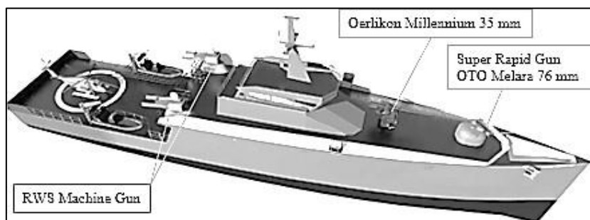
Fig.2. 3D Patrol Ship Design [3]
