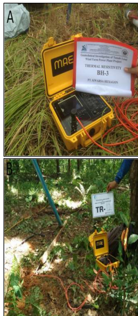
Figure 4. Thermal resistivity measurement at (A) BH-03 at Sapu Angin hill, sub-district Panyipatan and (B) BH-12 at Kampung Baru, sub-district Pelaihari.
