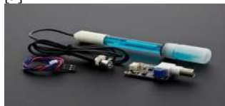
Gambar 1 Sensor pH SEN0161 [8]
